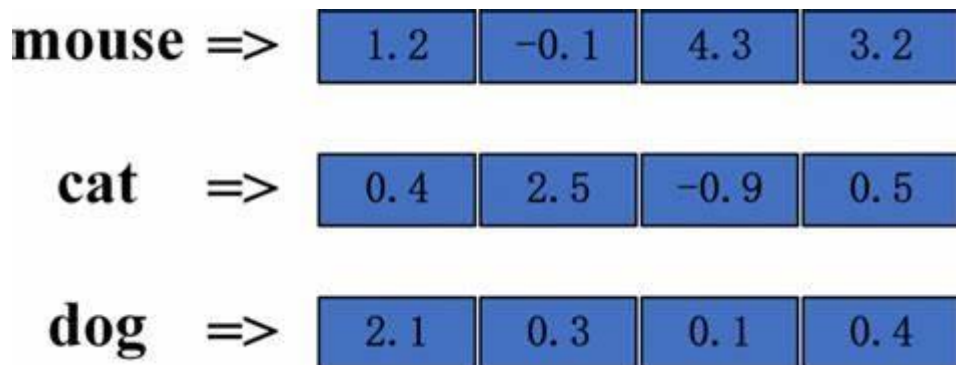
Figure 1.3: Transforming a word into a 4-dimensional vector
