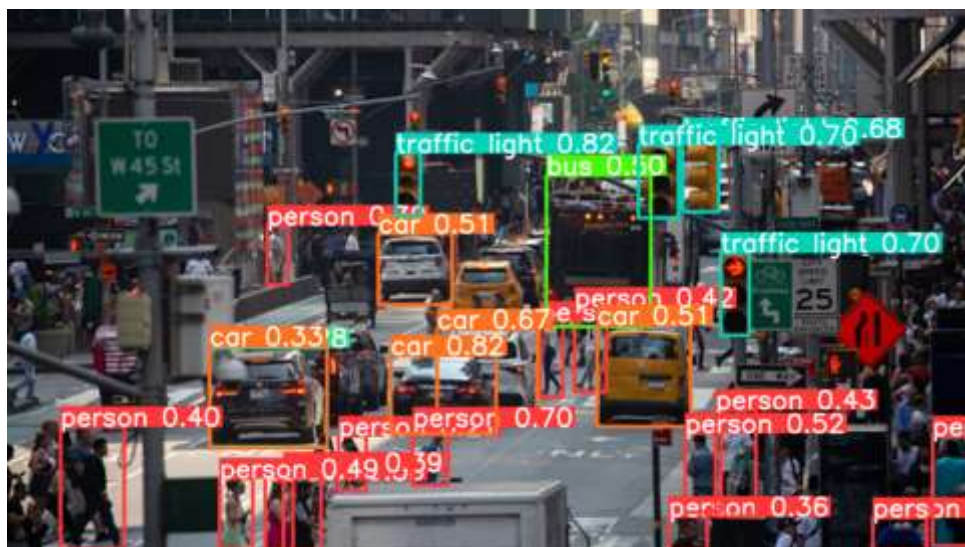
Figure 5.11 Object detection with YOLOv8.
