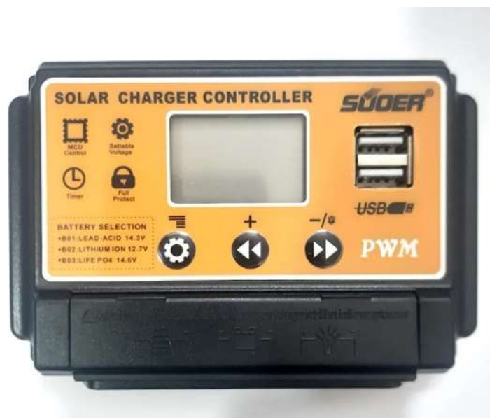
Figure 3–16: Solar charger controller [27]
