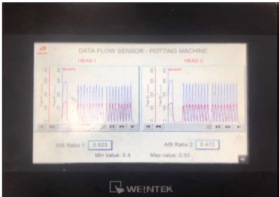
Figure 5.2 HMI screen displaying adhesive flow rate
