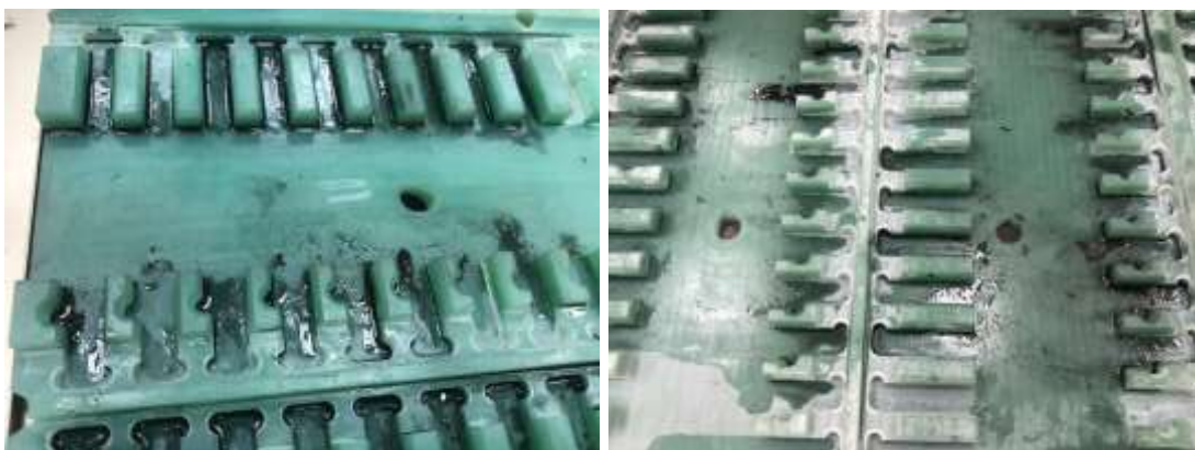
Figure 1.36 Glue sticking on the tool
