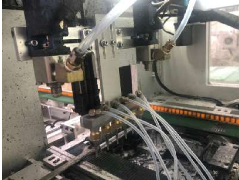
Figure 2.26 Install the glue splitter
