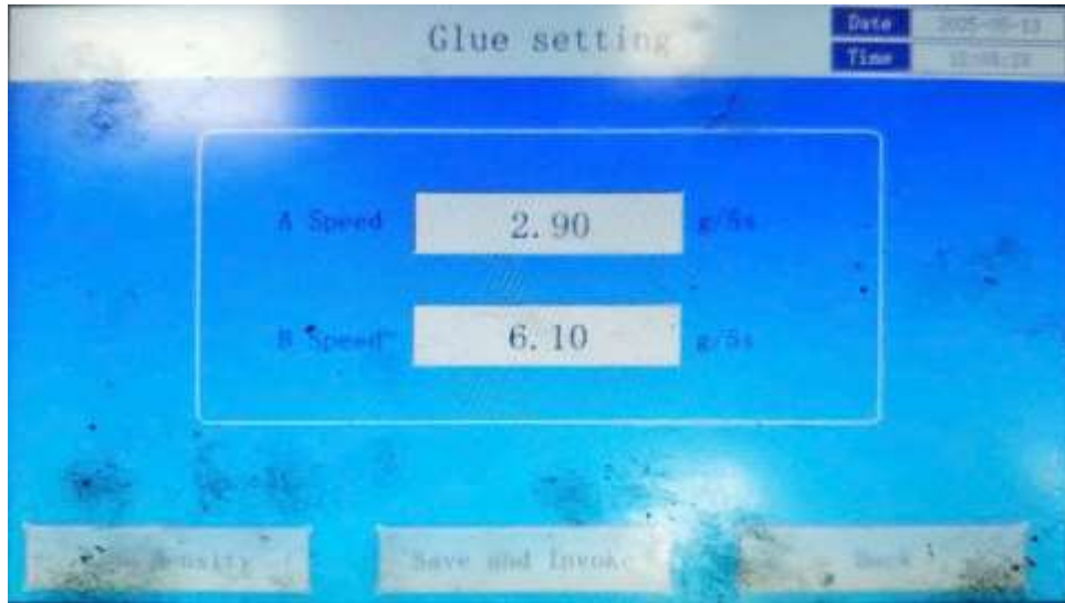
Figure 4.5 Flow rate setting and actual flow rate inspection
