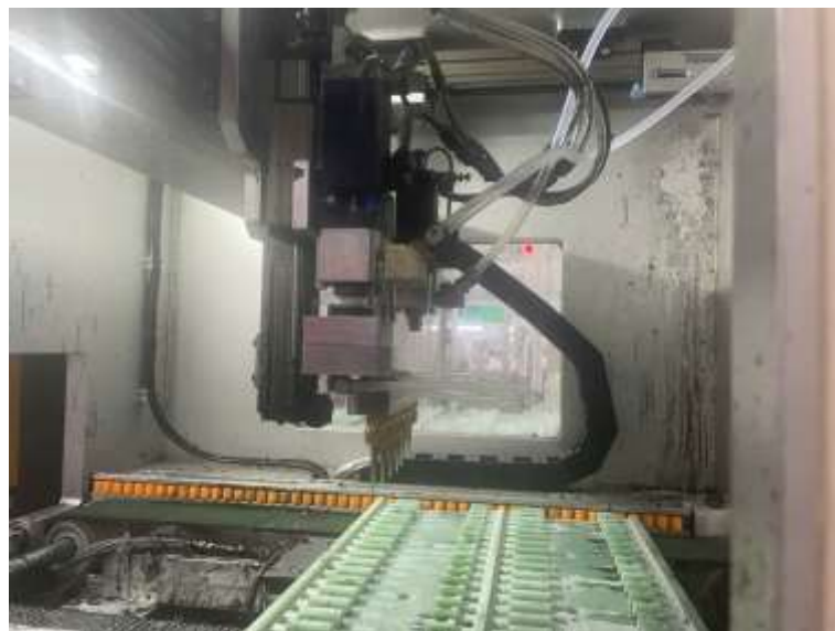
Figure 2.27 Overall view of the adhesive dispensing head tool system after installation
