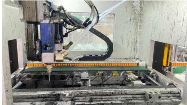
Figure 2.16 Two adhesive dispensing heads inside the potting machine
