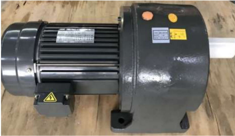
Figure 3.5 TDT geared motor driving chain transmission[Source: Internet]
