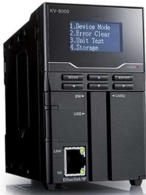
Figure 3.2 PLC keyence kv 8000
