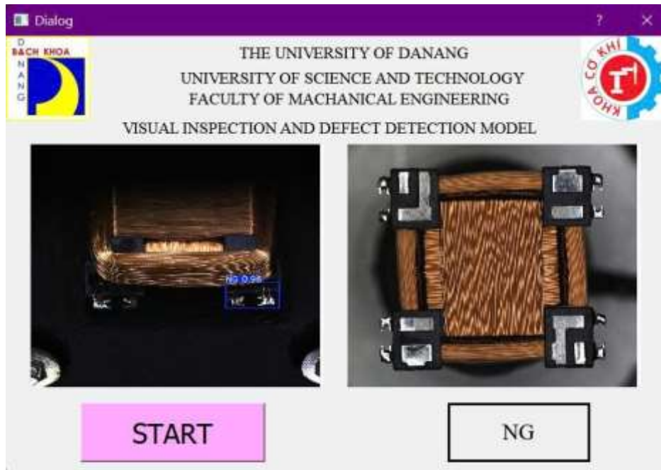
Figure 4.6. GUI Display Result of Defect Inspection for Product Not Meeting Requirements
