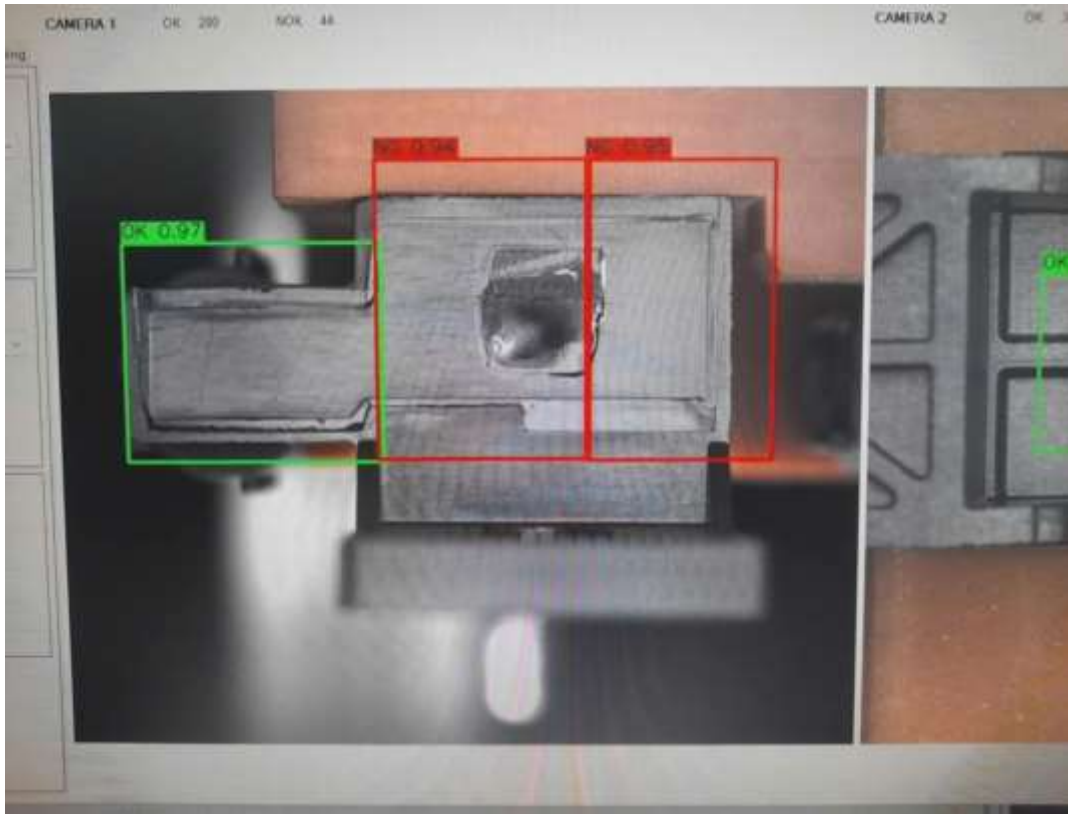
Figure 4.8. Actual defect inspection results for NG (non-conforming) casted parts (image 2)
