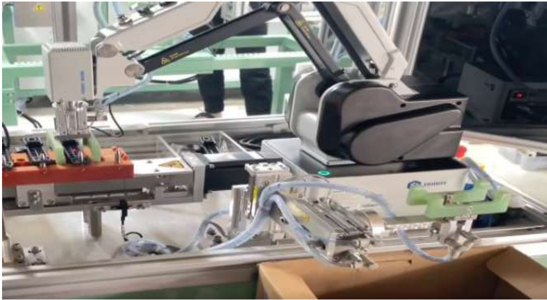
Figure 3.3. Sorting cast parts with Dobot after defect detection
