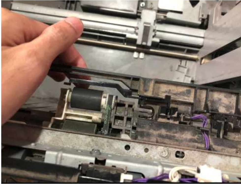
Figure 2.18 Paper picking mechanism of the trays
