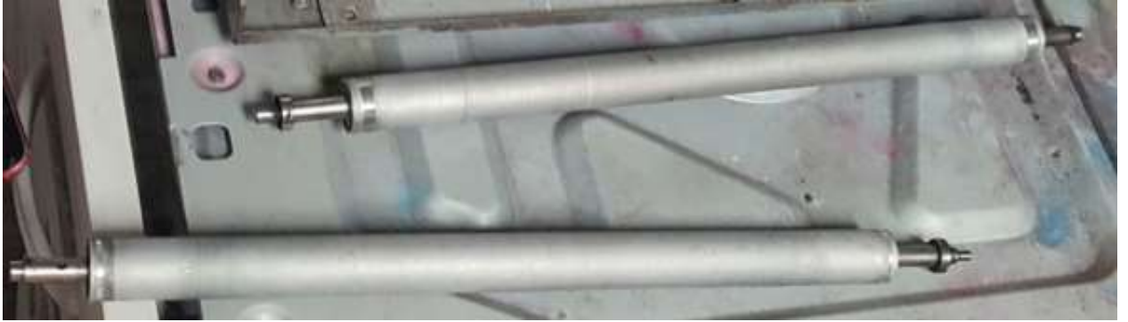
Figure 2.27 Rotary shaft used for the conveyor belt
