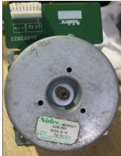
Figure 3.38 Brushless DC motor specifications from the manufacturer Accordingly, this motor has a power output of 28.1 W.
