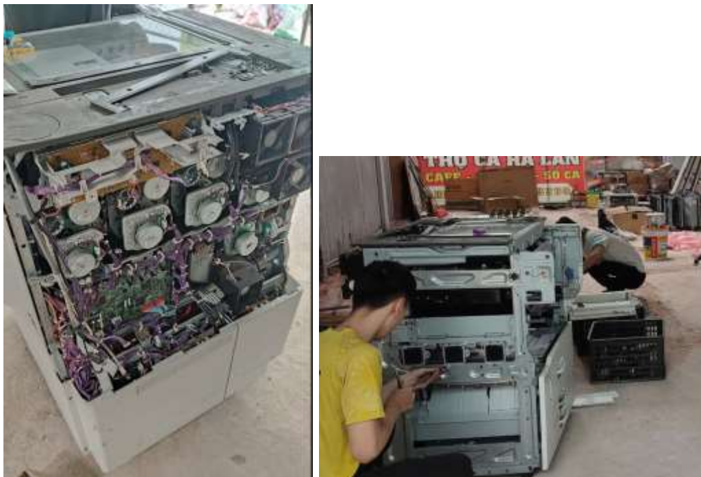
Figures 2.19 Disassembly of components on the printer
