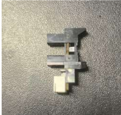
Figure 3.1 U-shaped photoelectric sensor
