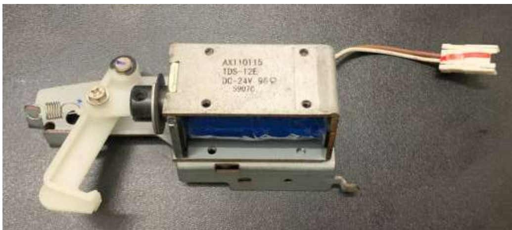
Figure 3.26 Electromagnet in the paper picking assembly
