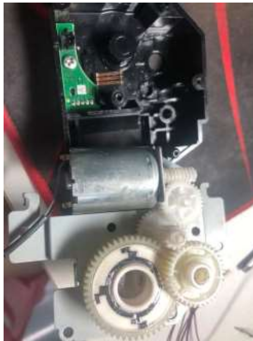
Figure 3.19 Internal structure of the motor
