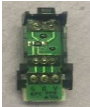
Figure 3.2 Structure and pin diagram of the U-shaped photoelectric sensor
