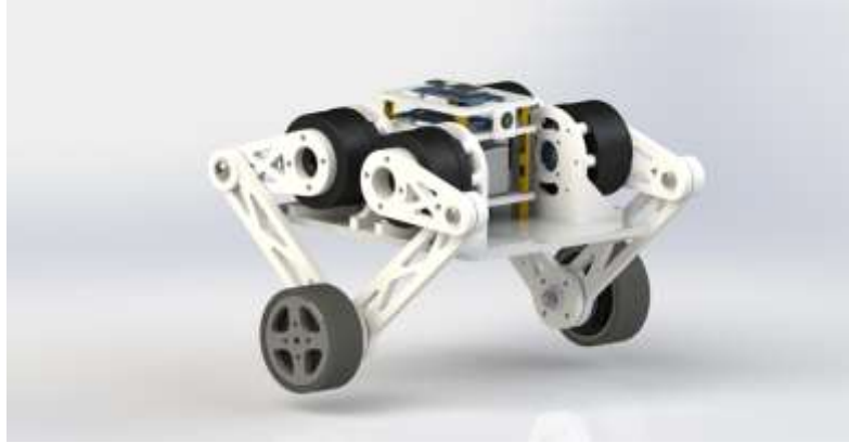
Hình 2.10 The shape of the robot with Option 1, a 5-bar linkage design
