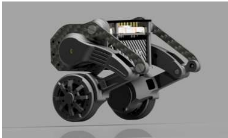
Figure 2.11 The shape of the robot with Option 2, a 4-bar mechanism type
