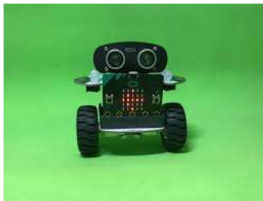
Figure 1.3 Two-wheel balancing robot using PID
