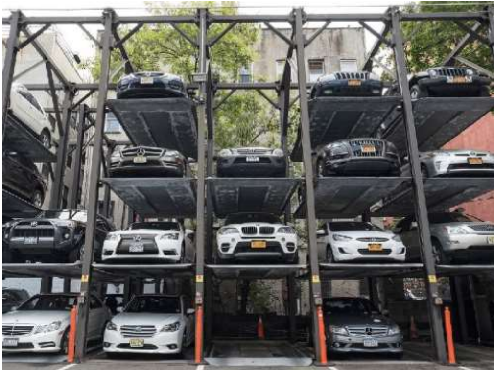
Figure 2.4 Modular Mechanical Parking System
