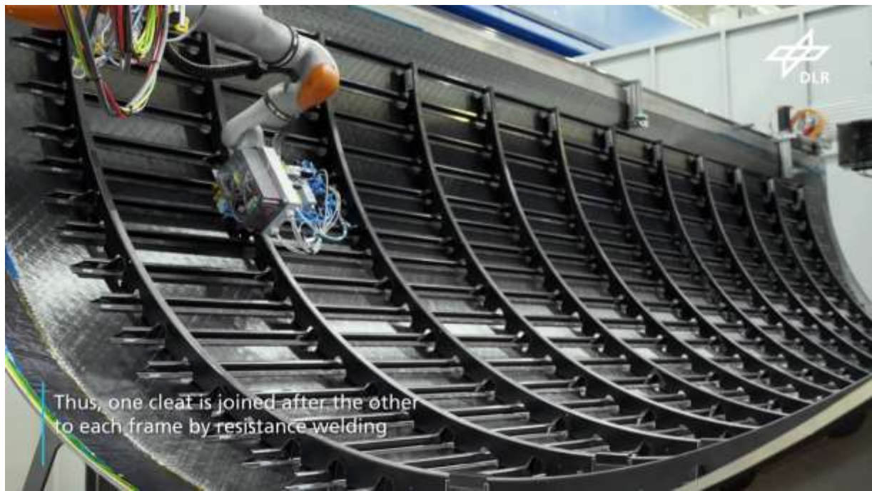
Figure 4. 16 Production of composite fuselage frame assemblies
