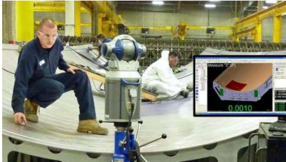
Figure 5. 15 Using a Laser Tracker to measure the aircraft fuselage
