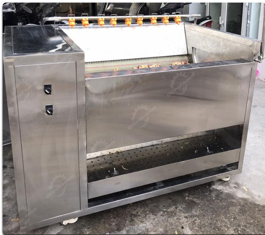
Figure 2. 3. Industrial Potatoes Washing Machine
