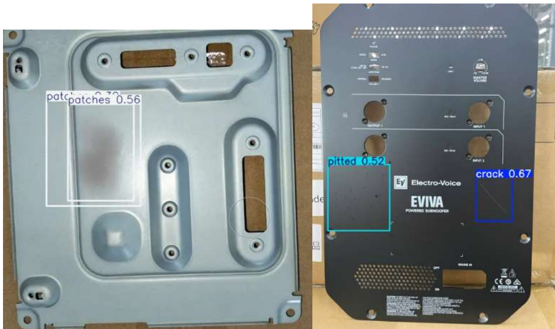
Figure 5.9 Examples of detection results.
