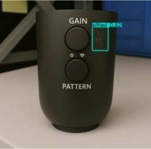
Figure 2.5 Model localizing a pitted
