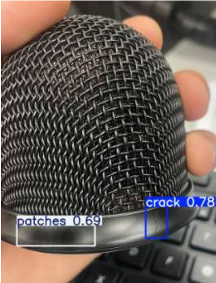
Figure 2.6 Model locating multiple defect types.
