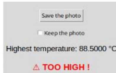
Figure 66 : GUI with visual overheat warning
