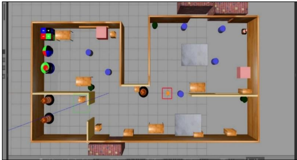
Figure 3.6: The Gazebo virtual environment for robot testing, this is the available package (the robot is in the red frame)
