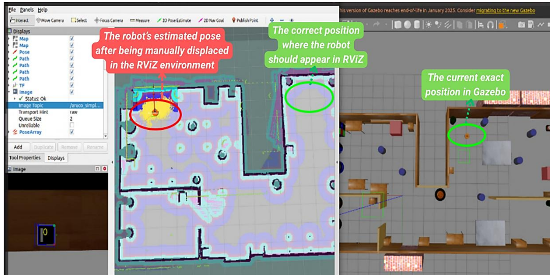
Figure 5.15: I used the Pose Estimate tool in RViz to manually displace the robot in Gazebo for testing the localization algorithm
