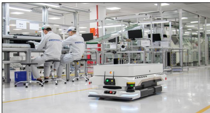
Figure 1.6: AMR at Phenikaa Electronics Factory (Source: AMR Autonomous Mobile Robot)
